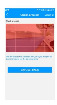
**6.4.4.Time setting for alarm information push :** It can set the time for the mobile phone to receive the alarm message push, taking 7 days as a cycle, and can be set to receive the alarm message at any time in a day.
