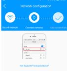
3.2. los:Click"next step"as the picture shows,The phone will switch to the WiFi list, Connected to the WiFi that starts with your device model, such as "JA-C6Kxxxx", the screen shown in picture appears, click it,then click"next step".
