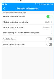
**6.4.1.Motion detection switch:** Select to turn the motion detection function on or off .
