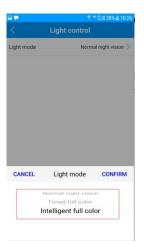
**6.8.1. Normal night vision:** In this mode, when the ambient brightness is low, the infrared light will be on, the white light will not be on, and the monitoring screen is black and white.
