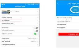
**6.3.1.Record mode:** The recording definition can be set in FHD mode and standard mode
